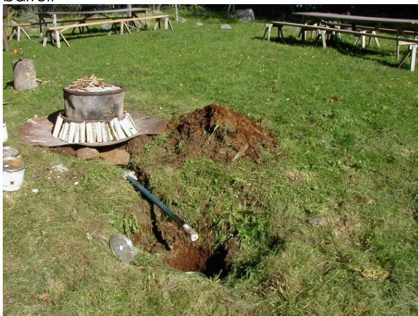
Here is the pipe where it will drop out about 5 liters Tar of good quality.
